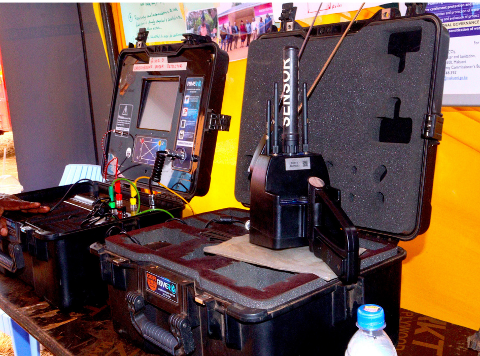
The digital River G underground water detector used by the Makueni borehole drilling unit for underground water detection
